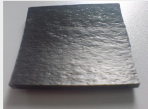
Figure 6: Fused granules create a rough structure on the lower surface of the polyamide top coat
