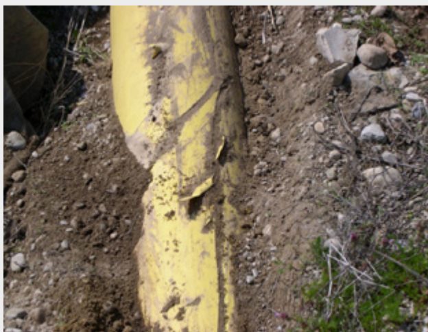
Figures 1 and 2: Damage caused by a digger tooth to a polyethylene-coated steel pipeline and a polyethylene pipeline
