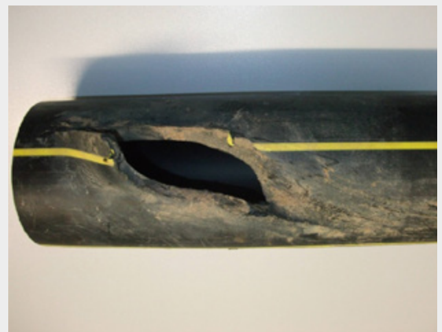
Figures 1 and 2: Damage caused by a digger tooth to a polyethylene-coated steel pipeline and a polyethylene pipeline
