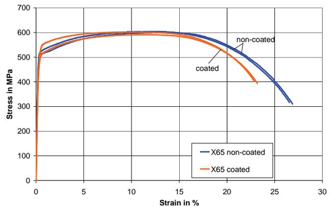
Figure 7: Tensile stress-strain curves (examples) of non-coated and coated pipes (grade X65, longitudinal test direction)
