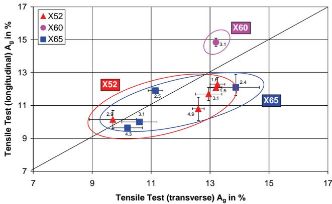
Figure 4: Comparison of uniform elongation  $A_g$  in tensile tests on round specimens taken in transverse and longitudinal direction as a function of the material grade (mean values and range)
