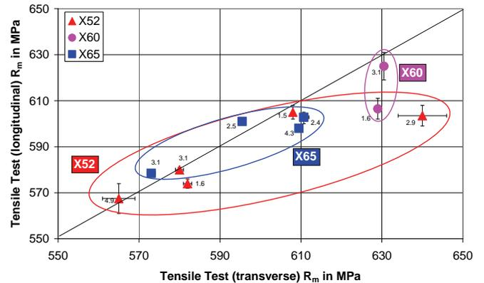
Figure 2: Comparison of tensile strength  $R_m$  in tensile tests on round specimens taken in transverse and longitudinal direction as a function of the material grade (mean values and range)
