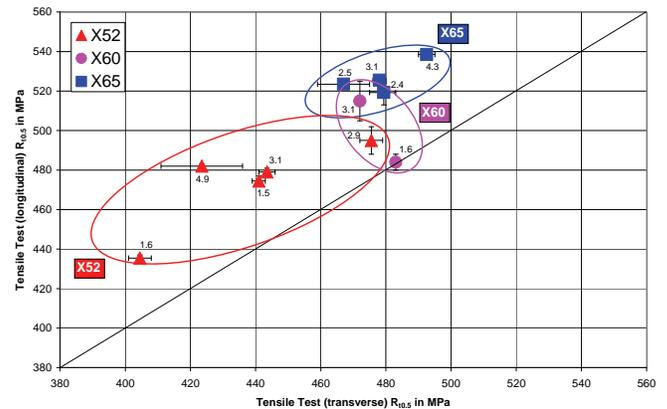
Figure 1: Comparison of yield strength  $R_{10.5}$  in tensile tests on round specimens taken in transverse and longitudinal direction as a function of the material grade (mean values and range)
