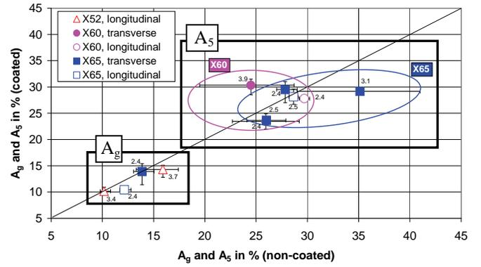
Figure 11: Comparison of  $A_g$  and  $A_5$  between non-coated and coated pipe as a function of the material grade and specimen orientation
