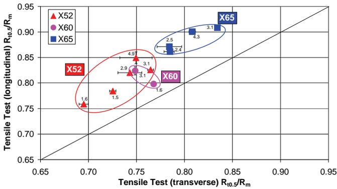
Figure 3: Comparison of yield-to-tensile ratio  $R_{t0.5}/R_m$  in tensile tests on round specimens taken in transverse and longitudinal direction as a function of the material grade (mean values and range)
