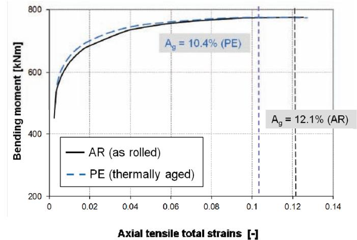
Figure 12: Bending moment – strain evolution for the tensile zone
