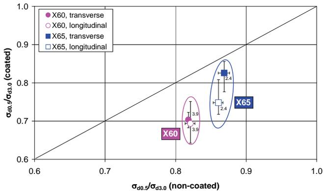
Figure 10: Comparison of  $\sigma_{d0.5}/\sigma_{d3.0}$  between non-coated and coated pipe as a function of the material grade and specimen orientation
