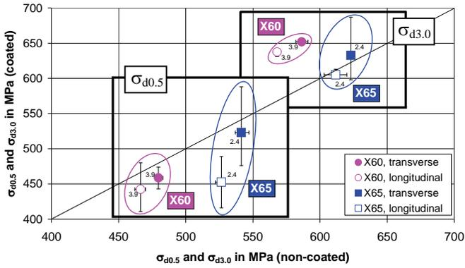
Figure 8: Comparison of  $\sigma_{d0.5}$  and  $\sigma_{d3.0}$  between non-coated and coated pipe as a function of the material grade and specimen orientation
