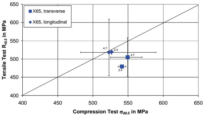
Figure 5: Comparison of yield strength in tensile ( $R_{t0.5}$ ) and compression ( $\sigma_{d0.5}$ ) tests on round specimens taken in transverse and longitudinal direction of the material grade X65 (mean values and range)
