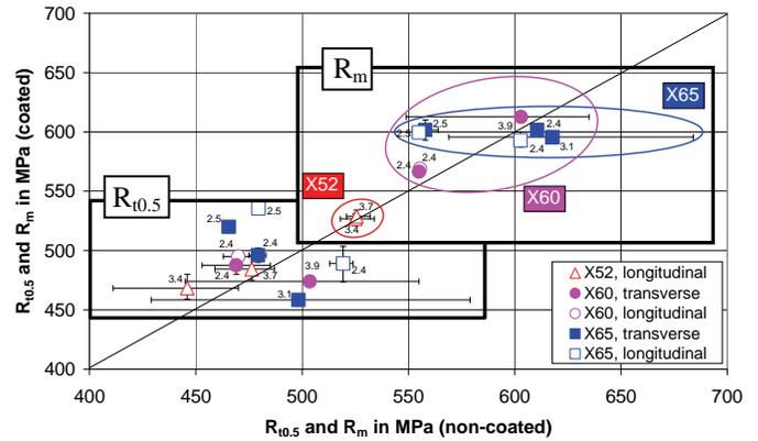
Figure 6: Comparison of  $R_{t0.5}$  and  $R_m$  between non-coated and coated pipe as a function of the material grade and specimen orientation
