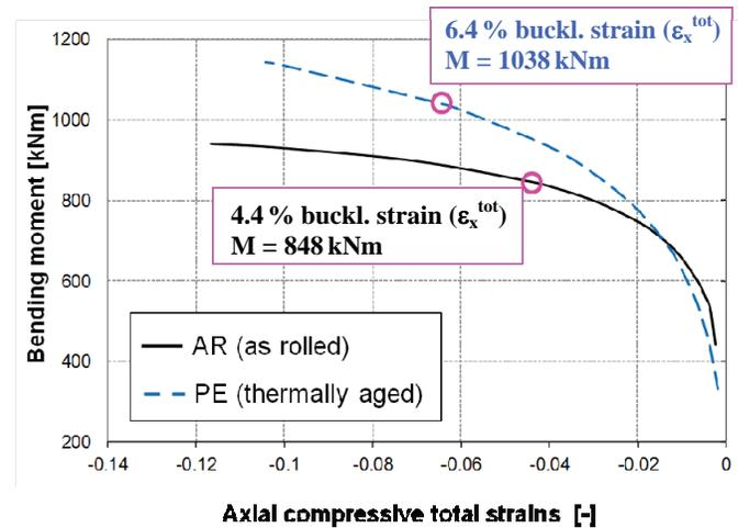
Figure 13: Bending moment – strain evolution for the compression zone
