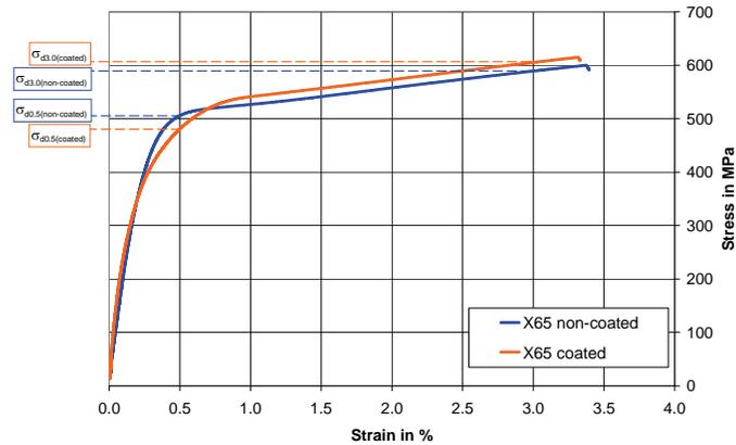
Figure 9: Compressive stress-strain curves (examples) of non-coated and coated pipe (grade X65, longitudinal test direction)
