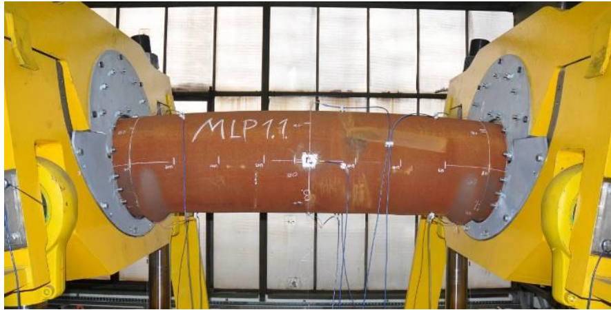
Figure 3: Pipe deformation after test, with buckles next to the clamping supports
